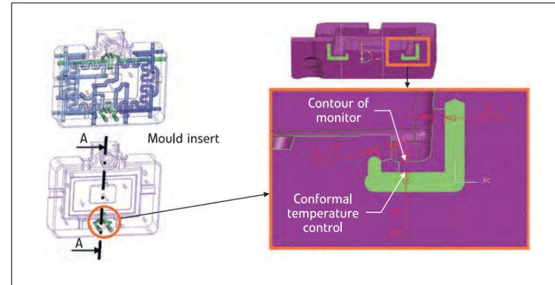
Fig. 3. The conformal mould cooling conceals the weld in the exposed high-gloss area
