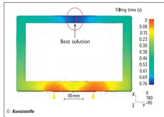
Fig. 2. Position of the welds with optimised gating
