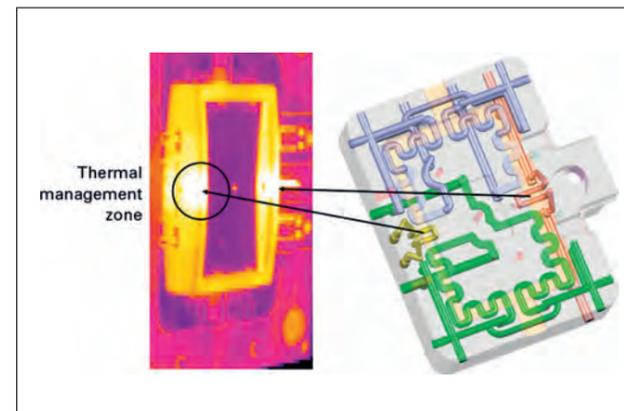
Fig. 5. Infrared thermograph of the mould insert for thermal management
