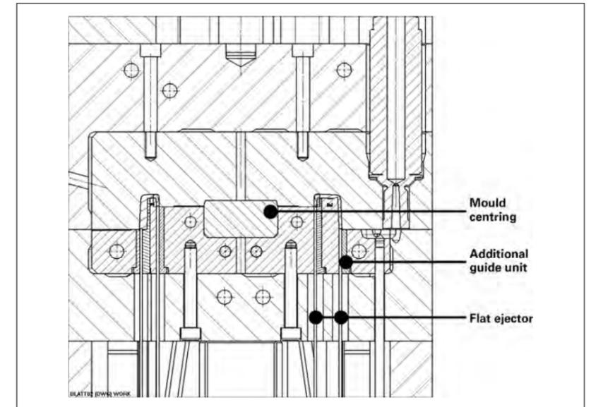
Fig. 4. Section view through the mould with flat ejector, including centring
